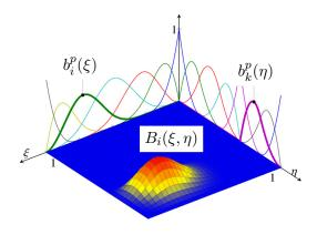
**Properties**: compact support, positive function values, partition of unity  $\sum\limits_{i=1}^{n}B_{i}(\xi,\eta)\equiv 1$ ,  $C^{p-1}$  continuity, derivatives of B-splines are combinations of lower-order B-splines, ...
