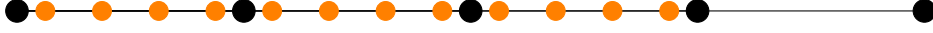
Figure 3.2: Discretized domain \Omega \in \mathbb{R} and initial configuration \Omega_0 \in \mathbb{R} consisting of five degrees of freedom and equally distributed particles.
