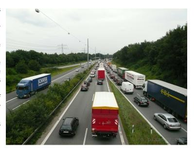
We have developed a lane distribution model describes and predict how a flow of different types of vehicles (e.g. cars and trucks) would distribute itself over the multiple lanes of a freeway (e.g. only trucks on the outer lane and only cars on the other 2 lanes, or cars on all lanes, but mixed with trucks on the outer 1 or 2 lanes). So far, the lane distribution model has only been developed for very simple static problems.
